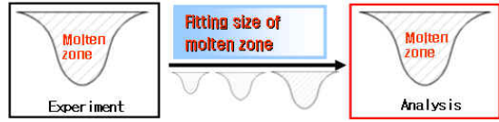
(b) changing the maximum intensity of the heat source, Q_0 and Q_1
